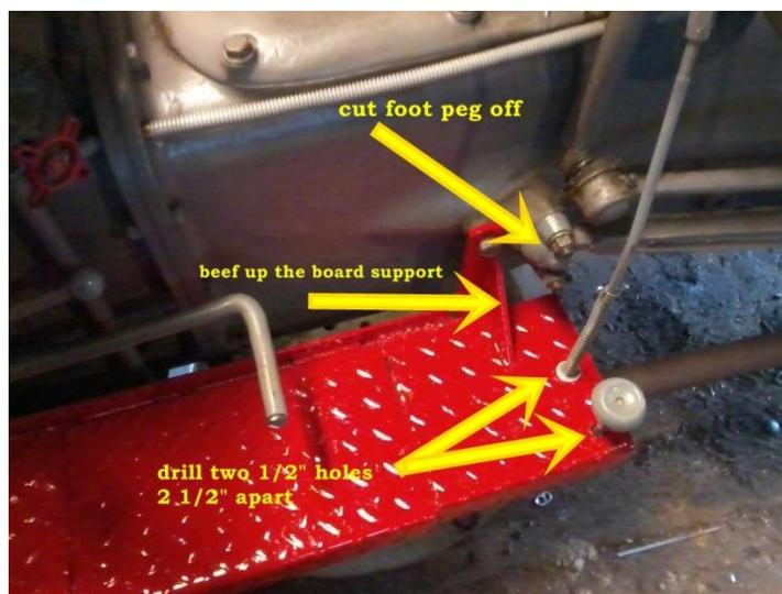
First you will need to cut off the foot peg. It is in the way of where the new linkage will be moved to. My floor board had a brace that hung off the foot peg for added support; I had to cut it off. I used that steel to beef up the brace that bolts to the tractor. Next you will need to drill two ½" holes for the throttle linkage to pass through. They don't have to be perfect but you do need to remove any burrs that could cause it to bind. 1" in from the edge and 2 ½" apart.
