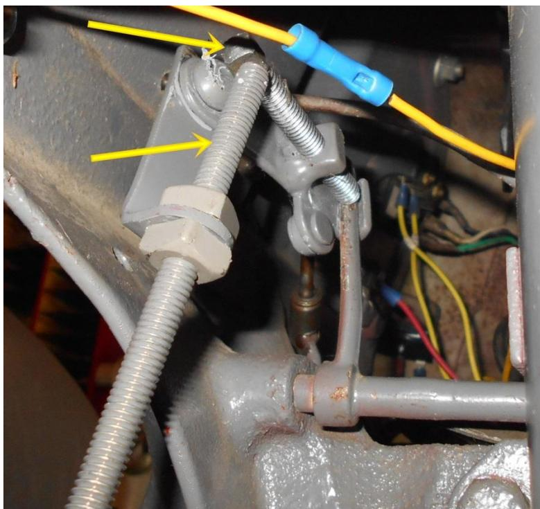
My kit was missing the bolt, instead of waiting for them to send me one I just made one. You will need to use 5/16" x 18tpi threaded rod and a coupler to extend the Dowden linkage because the foot feed is mounted lower and therefore is farther away. The threaded rod in this
